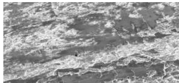
Fig.6: SEM Image for 1 hour hardened specimen
